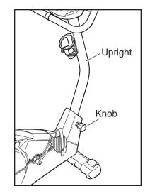
the knob. Move the upright up and down slightly until the pin on the knob snaps into one of the holes in the upright. Then, turn the knob clockwise until it is tight.
